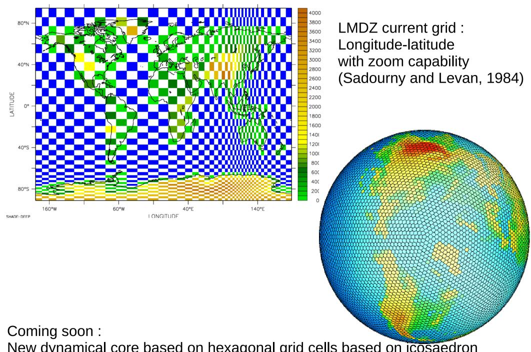
New dynamical core based on hexagonal grid cells based on icosaedron (Dubos, Meurdesoif et al. 2016)
