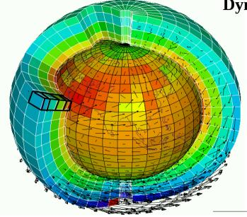
Dynamical core: primitive equations discretized on the sphere
