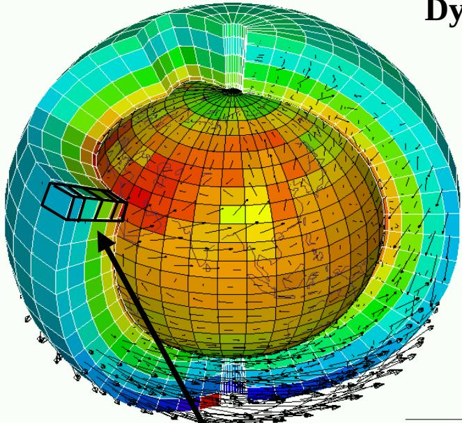
Dynamical core : primitive equations discretized on the sphere
