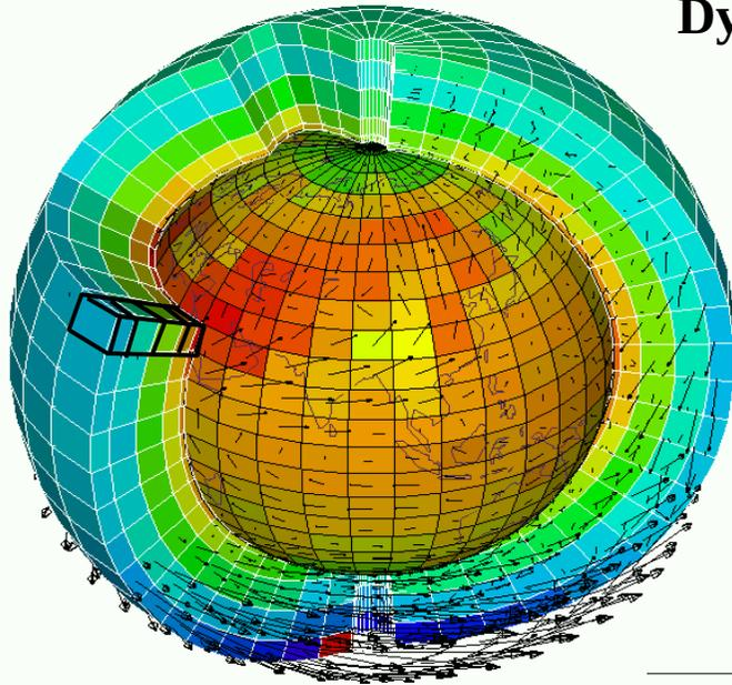
**Dynamical core : primitive equations discretized on the sphere**
