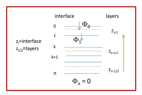
• Bottom :  $\Phi_n$  = 0  $T_{n-1/2}^t = \alpha_{n-1}^t \ T_{n-\frac{3}{2}}^t + \beta_{n-1}^t$
