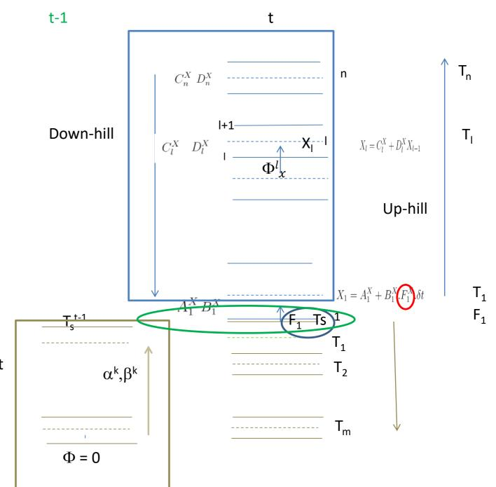
At t  $\alpha_k$  and  $\beta_\kappa$  depend on  $T_k$  at the previous time step and on the underlying layers : They can be pre-computed
