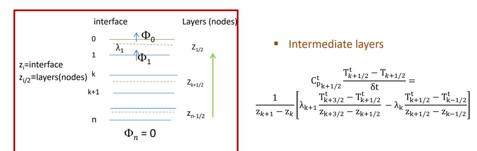
$$C_{p_{k+1/2}}^{t} \frac{T_{k+1/2}^{t} - T_{k+1/2}}{\delta t} = \frac{1}{z_{k+1} - z_{k}} \left[ \lambda_{k+1} \frac{T_{k+3/2}^{t} - T_{k+1/2}^{t}}{z_{k+3/2} - z_{k+1/2}} - \lambda_{k} \frac{T_{k+1/2}^{t} - T_{k-1/2}^{t}}{z_{k+1/2} - z_{k-1/2}} \right]$$
