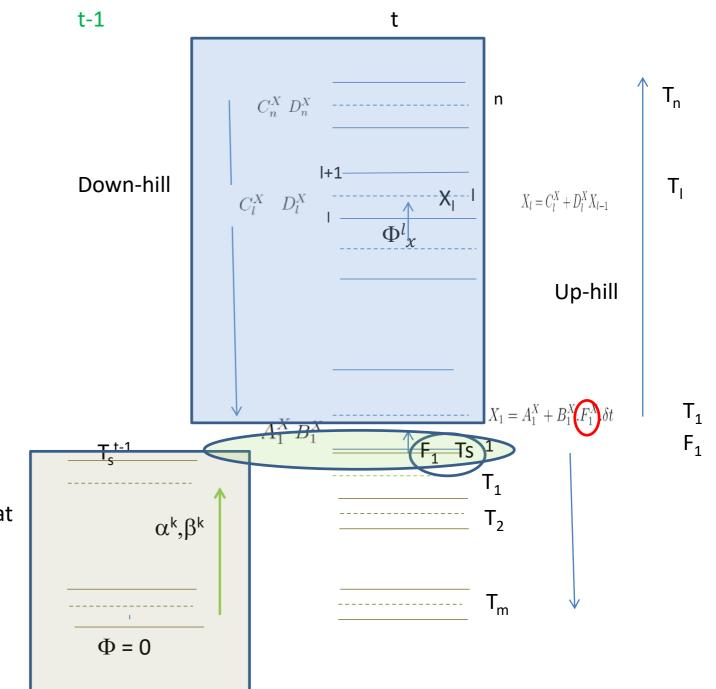
At t  $\alpha_k$  and  $\beta_\kappa$  depend on  $T_k$  at the previous time step and on the underlying layers : They can be pre-computed
