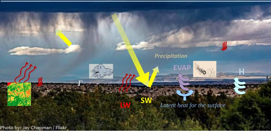
The **atmosphere and the surface are coupled** through *turbulence* (in boundary layer) and *radiation*
