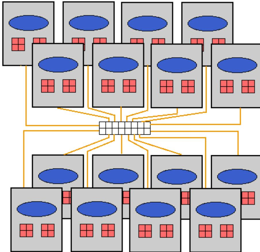
Example of a cluster of **16 nodes** with **32 cpus** and **128 cores**
